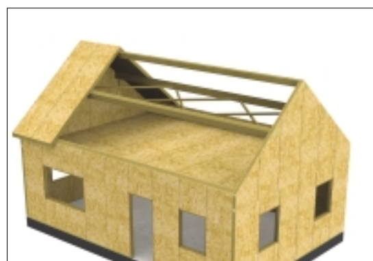
Figure 29b FIRST OPPOSING PAIR OF ROOF SECTIONS INSTALLED
